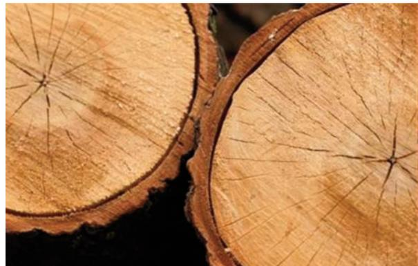
The wood humidity is approx. 7-10% at the time production is complete. During the subsequent natural drying process of solid wood, small hairline cracks (particularly around branches) are unavoidable. These are practically invisible with non-stain treatments, treatment with wood tones or un treated products. However, these cracks may become visible under opaque surface treatments. Unfortunately this is unavoidable.
